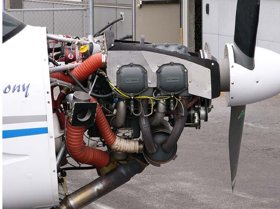
A Lycoming O-320-D2A installed in a Symphony SA-160 By Ahunt at English Wikipedia, Public Domain https://commons.wikimedia.org/w/index.php?curid=8015248
