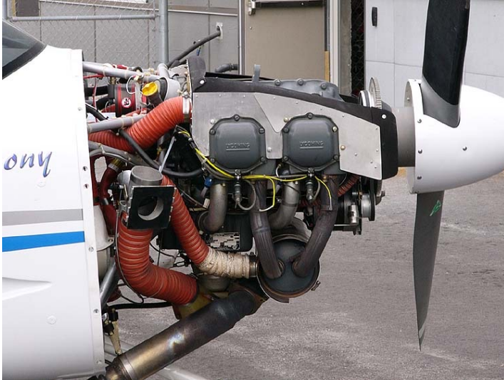
A Lycoming O-320-D2A installed in a Symphony SA-160
